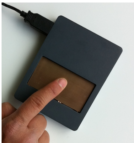
Figure 1.8 – The Stimtac device produces a variable friction haptic feedback.
