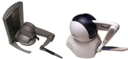
Figure 2 – PHANToM Desktop et OMNI
