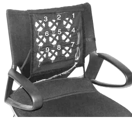
Figure 27 – Le haptic back display
