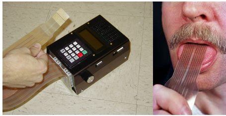
Figure 18 – Tongue Display Unit
