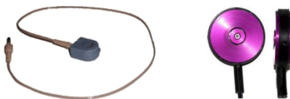
Figure 26 – Tactor VBW32 et C2
