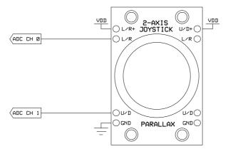
This circuit creates two voltage dividers referenced to VDD (in this case 5 V), using a 2-channel ADC (in this case the MCP3202) to read the voltages at the L/R and U/D pins using the code below. **Caution:** Do not apply voltage to the L/R+ or U/D+ pins that exceeds the I/O pin voltage rating of the device you connect to L/R or U/D, up to 10 VDC maximum. Ground<Analog voltage output at L/R and U/D<VDD.
